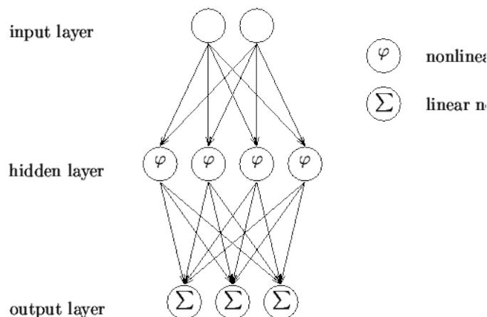
**Figure 2:** Signal-flow graph of an MLP
